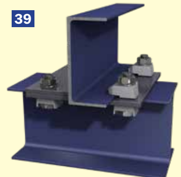
Channel positioned above I-Section at 90 degrees
