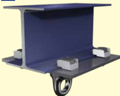
Fixed rigging point below an I-Section
